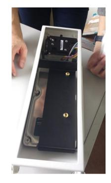
Fig. 1. Campbell Scientific CS110 Electric Field Meter Sensor
