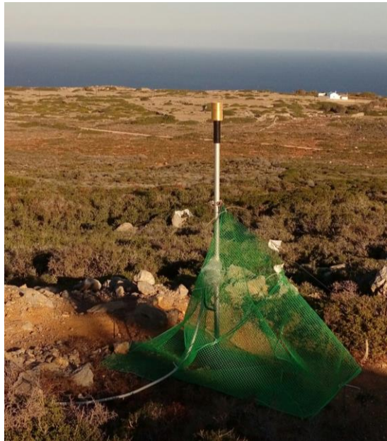
Figure 4: The electric field mill belonging to UH as installed at the field station on Antikythera. For security reasons a low fence comprised totally of plastic material surrounded the instrument.
